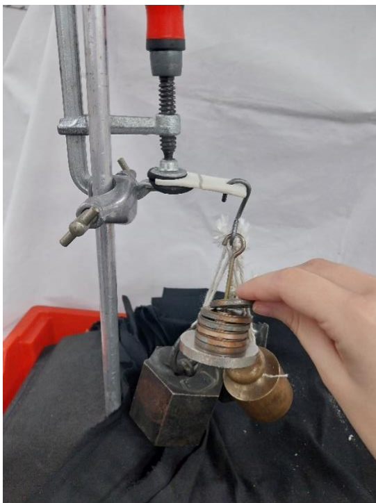
Figure 4 The researcher adding a weight to a clamped porcelain tile.
