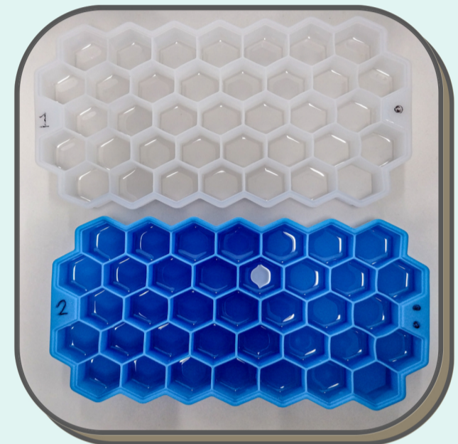
Fig. 1. Resin samples prepared in silicone moulds
