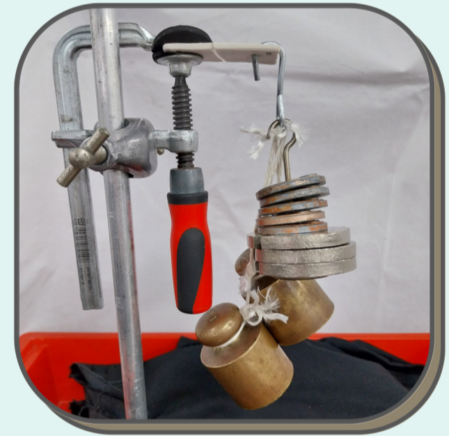
Fig. 2. Porcelain and adhesive strength testing
